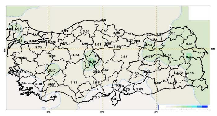
Fig. 3.1.1.7 00 UTC RMSE Values of Mean Sea Level Pressure for D+7
