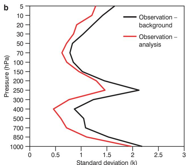
**Figure 6** (a) The Swedish icebreaker Oden from which temperature soundings were made in polar regions. (b) Comparison between ECMWF operational assimilation and temperature sounding data during a three-week period (1 to 22 August 2001) when Oden was anchored to the drifting sea ice very close to the north pole. The two curves show the standard deviation of temperature differences (K) between observations and analysis (red line) and observations and background (black line).
