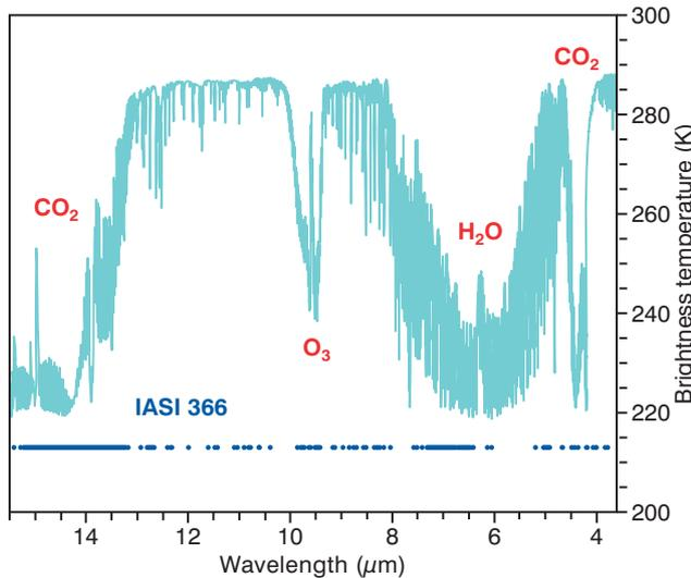
**Figure 1** The location of the processed IASI channels in the infrared spectrum. Note the large concentration of channels in the 15 μm CO<sub>2</sub> band region.
