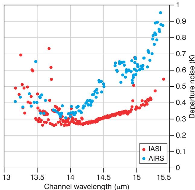
**Figure 2** Standard deviations of globally averaged observed minus computed radiance departure for the infrared long-wave band. The improved performance of IASI compared to AIRS in channels with wavelengths greater than 14 μm can be seen.
