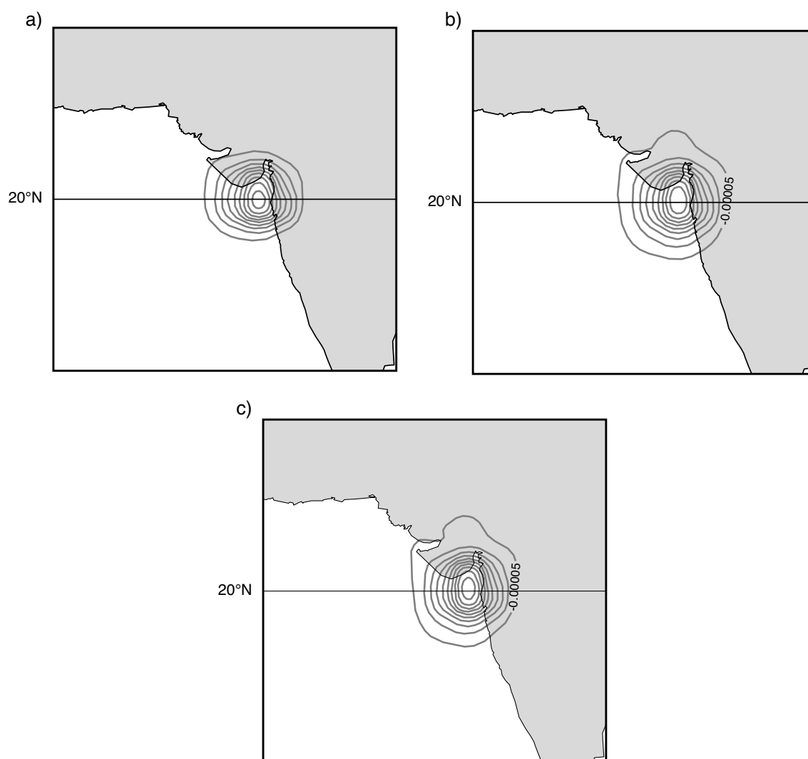
Figure 3: The specific humidity increments at model level 47 with the 1D operator (a), the 2D operator described in section 3.1 (b) and the 2D operator described in section 3.2 (c). The contour lines have a 5 \times 10^{-5} Kg/Kg interval.
