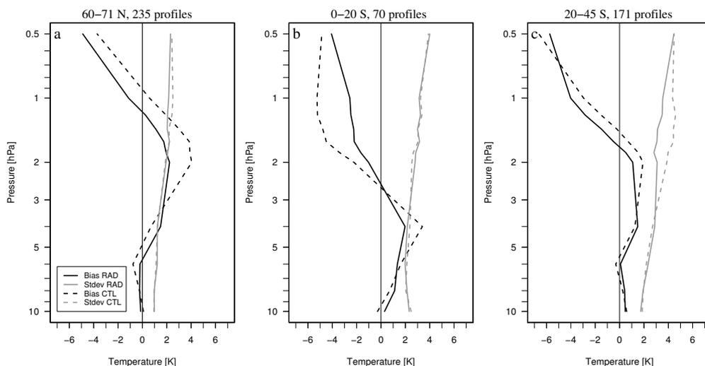
Figure 13: a) Statistics for differences between HALOE temperature retrievals and analyses [K]. Black lines indicate HALOE minus analysis biases, grey lines show standard deviations of the differences. Solid lines are for statistics for analyses from the RAD experiment, whereas dashed lines show statistics for the CTL analyses. Data cover the period 1-29 September 2003 and the north polar region. b) As a), but for the southern tropics. c) As a), but for the southern mid-latitudes.
