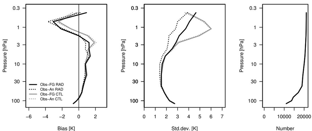
Figure 10: Departure statistics for MIPAS temperature retrievals (global) for 1-29 September 2003. Solid lines indicate statistics for FG departures, dotted lines statistics for analysis departures. Statistics for the RAD experiment are in black, for the CTL in grey. From left to right the three panels show the bias (retrieval minus FG or analysis), standard deviation, and the number of retrievals, respectively.
