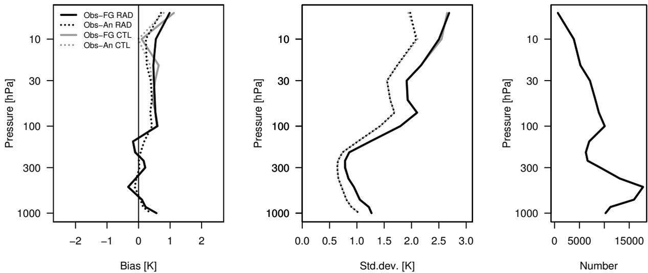
Figure 6: Departure statistics for used radiosonde temperature observations over the tropics for the period 1-29 September 2003. Solid lines indicate statistics for FG departures, dotted lines statistics for analysis departures. Statistics for the RAD experiment are in black, for the CTL experiment in grey. From left to right the three panels show the bias (sonde minus FG or analysis), standard deviation, and the number of observations, respectively.
