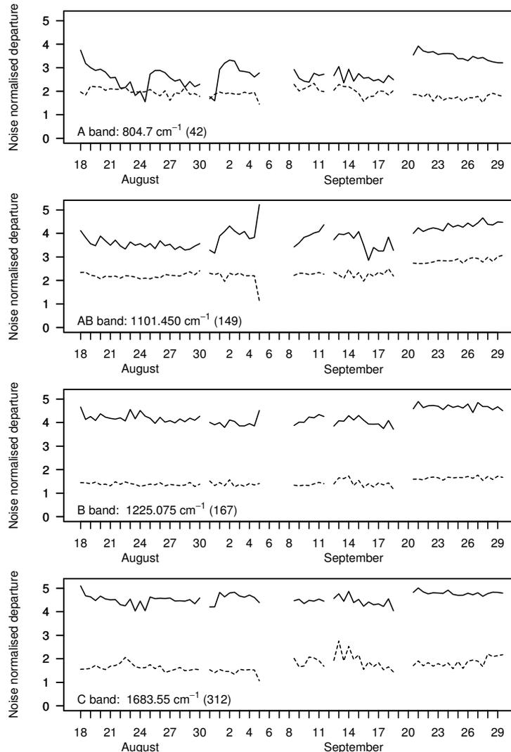
Figure 3: Time-series of global-mean observation minus FG biases (solid) and standard deviations (dashed) from the CTL experiment for four typical MIPAS channels, representative of the four MIPAS bands, as indicated in each panel. Numbers in brackets give the channel index as used in this study. Statistics are for data with a nominal tangent altitude of 27 km, and the bias has been normalised by the instrument noise. No correction of radiance biases has been applied.
