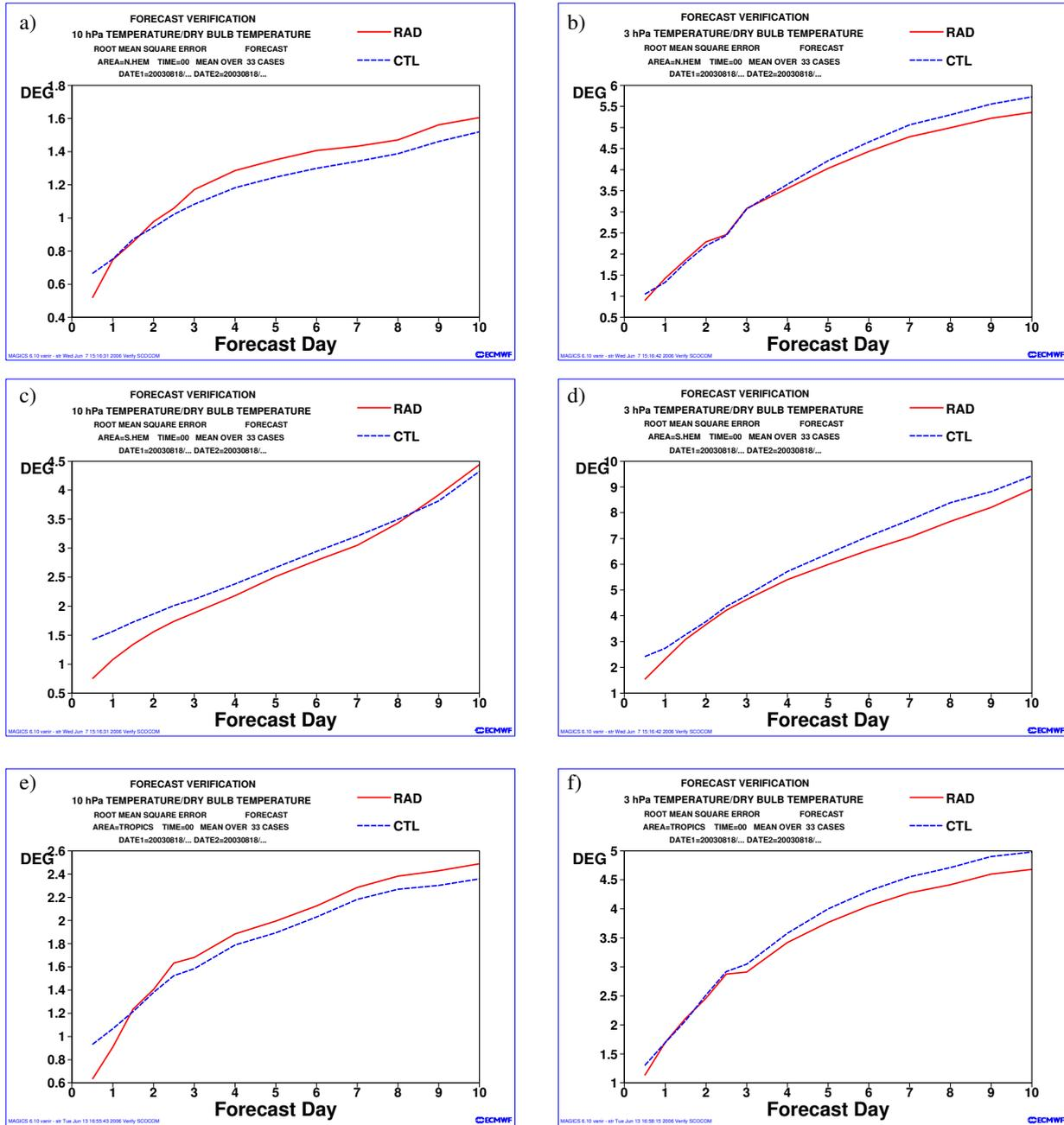
Figure 18: Root mean square errors for temperature forecasts from RAD (red solid) and CTL (blue dashed) as a function of forecast range. The panels show scores for the Northern Hemisphere (a, b), the Southern Hemisphere (c, d), and the Tropics (e, f) at 10 hPa (a, c, e) and 3 hPa (b, d, f).
