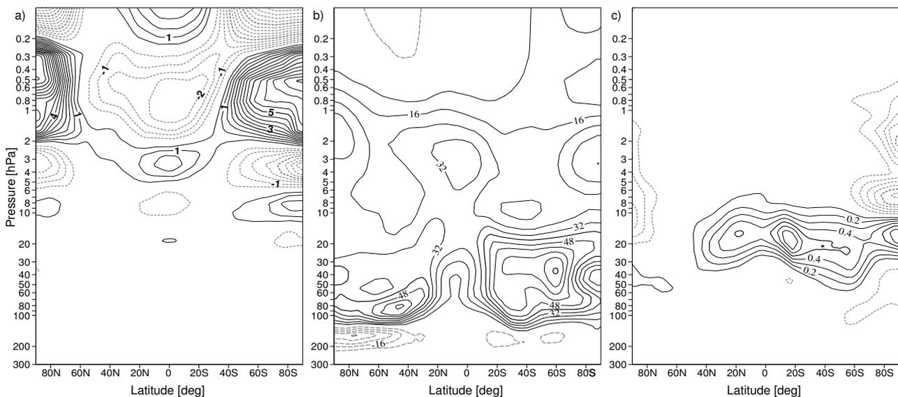
Figure 9: a) Zonal mean temperature differences between the experiments with and without assimilation of MIPAS radiances. Contour interval is 0.5 K, with positive values shown by solid black contour lines and negative values shown through dashed grey lines. b) Same as a), but for humidity (relative to the experiment without MIPAS radiance assimilation), with a contour interval of 8 %. c) Same as a), but for ozone volume mixing ratio with a contour interval of 0.1 ppmv.
