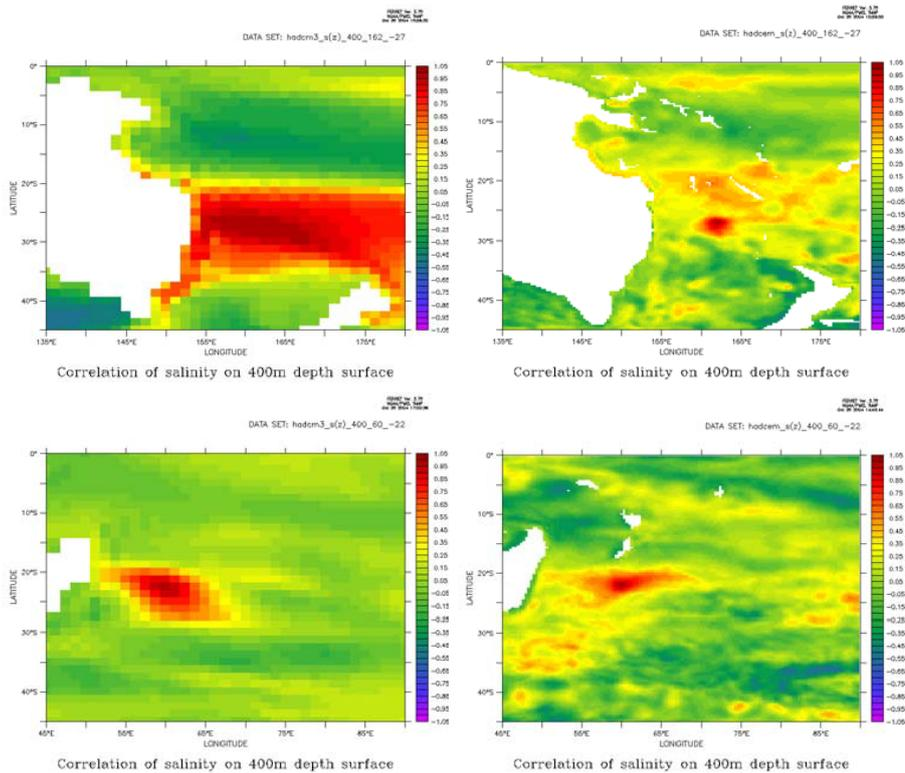
Figure 3: One-point correlation maps for  $S(z)$  at 400m. The left panels show results from 100 years of the low resolution climate model HadCM3, and the right panels show results from 10 years of the higher resolution HadCEM model at the same locations. The upper panels are located at 162E, 27S in the south Pacific off Australia, and the lower panels are located at 60E, 22S in the Indian Ocean east of Madagascar.
