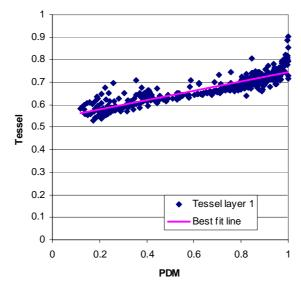
Figure 3: Scatter plot of PDM and Tessel estimates of relative soil moisture for the Mole.
