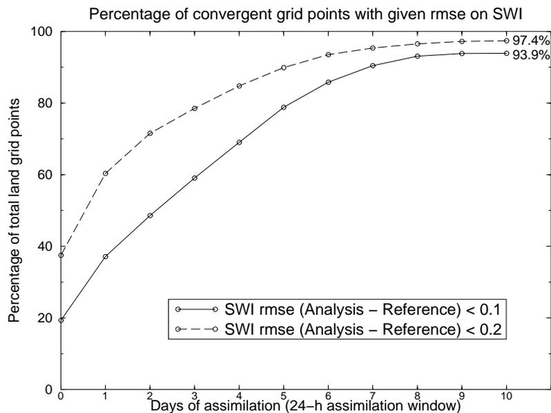
Figure 1: Convergence of 2D-VAR towards  $W_p^{ref}$ . Sequential assimilation with 24-h time-window (simulated observations every 6-h) starting the 13th June 2000. Percentage of total land grid points converging with given rmse on SWI; continuous line:  $rmse < 0.1$ , dashed line:  $rmse < 0.2$ .
