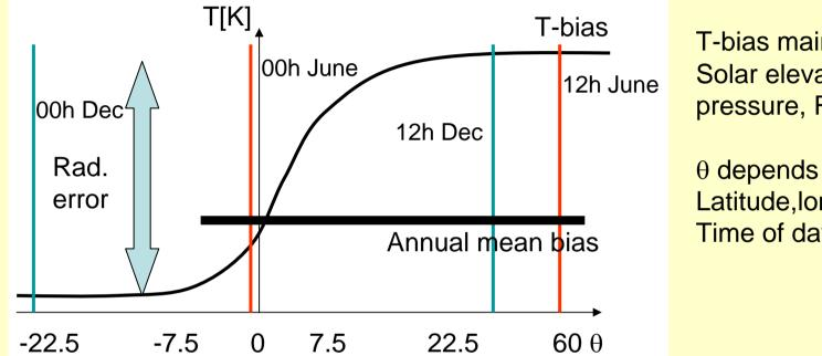
T-bias mainly a function of Solar elevation angle  $\theta$ , pressure, RS-type
