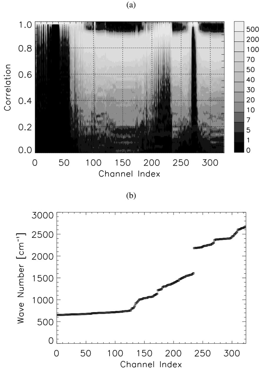
Figure 3: Figure (a) presents the bi-dimensional histogram of the correlation between linear and non-linear brightness temperature perturbations for each one of the 324 AIRS channel subset. The input temperature and humidity perturbations follow the statistics of the ECMWF background error. Negative correlations are not represented. The correspondence between channel index and wave number is shown in Figure (b).
