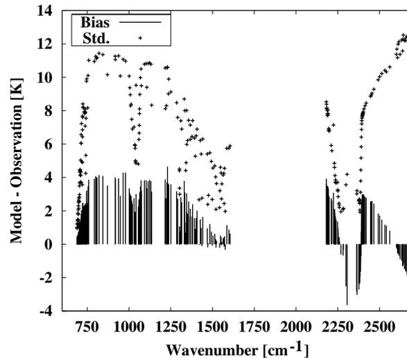
Figure 1: Bias and standard deviation of the differences between the model and the cloud-affected observed AIRS brightness temperatures on 30 November 2002. The model uses the prognostic cloud scheme. Above  $2000 \text{ cm}^{-1}$  day-time pixels are discarded.
