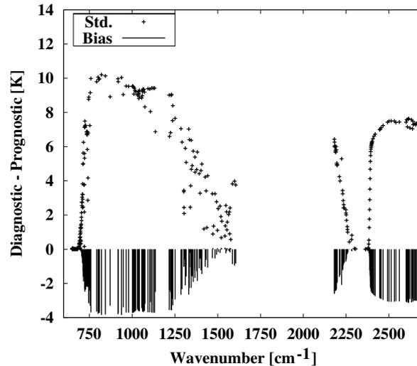
Figure 2: Bias and standard deviation of the differences between the model diagnostic and prognostic AIRS brightness temperatures. Model data correspond the Meteosat-7 disk on 30 November 2002 at 12 UTC. Clear points are removed using the Meteosat-7 cloud detection. In contrast to Figure 1, stratospheric channels are not removed.
