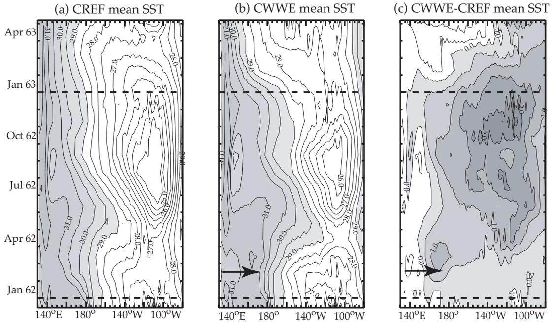
Figure 6: Equatorial sections of ensemble-mean SST simulated by the coupled model (CREF) and when inserting the March 1997 westerly wind event (indicated by the arrow, CWWE), and their difference.
