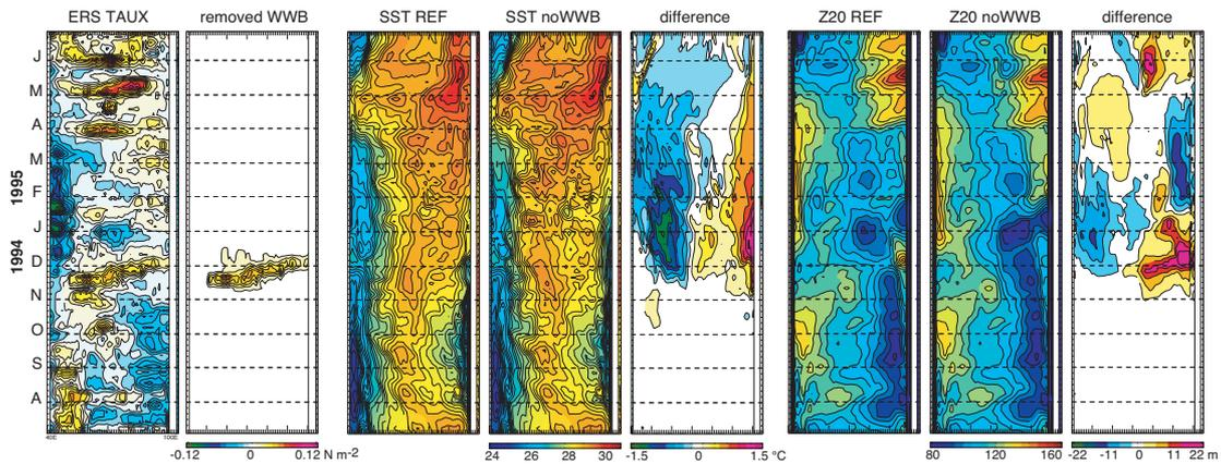
Figure 1: From left to right,  $2^{\circ}\text{N}$ - $2^{\circ}\text{S}$  mean: zonal wind stress from ERS data, westerly wind stress pattern from ERS data, SST simulated by OPA, SST simulated by OPA when forcing without the westerly wind stress pattern, SST difference between the two simulations, simulated  $20^{\circ}\text{C}$  isotherm depth, simulated  $20^{\circ}\text{C}$  isotherm depth when forcing without the westerly wind stress pattern,  $20^{\circ}\text{C}$  isotherm depth difference.
