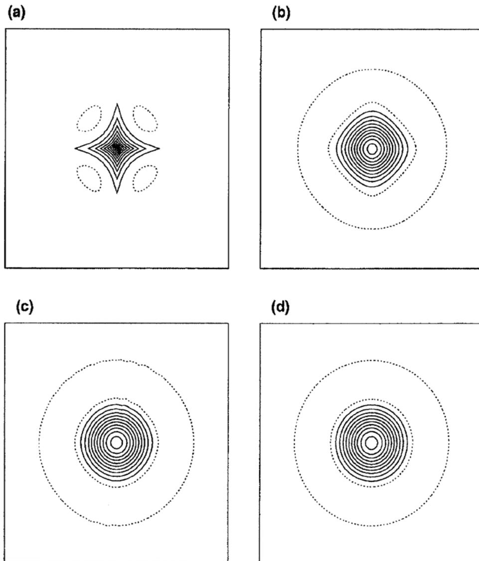
Figure 3: Negative Laplacian applied to quasi-Gaussian recursive filters with (a)  $n = 2$ , (b)  $n = 4$ , (c)  $n = 6$ , and (d) corresponding contours for the exact Gaussian. Contours are at multiples of odd numbers with negative contours shown as dotted curves. From Purser et al. (2003a).
