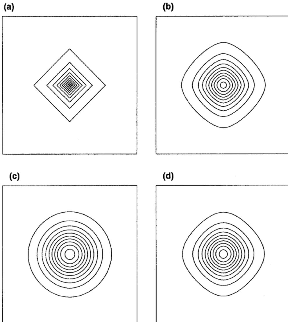
Figure 2: Sequential application of quasi-Gaussian recursive filters of order  $n$  in two dimensions (a)  $n = 1$ , (b)  $n = 2$ , (c)  $n = 4$  and (d) four applications of filters with  $n = 1$  with scale parameters adjusted to make the result comparable with the other single-pass filters. From Purser et al. (2003a).
