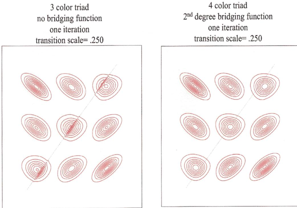
Figure 4: Correlation functions when strong (90°) transition in orientation over short distance. Left without bridging function. Right with bridging function.
