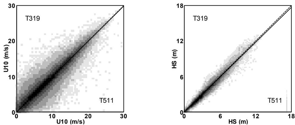
Figure 2 Comparison between the wind speeds (left panel) and the wave heights (right panel) obtained with different resolutions of the meteorological model, T319 vs T511.
