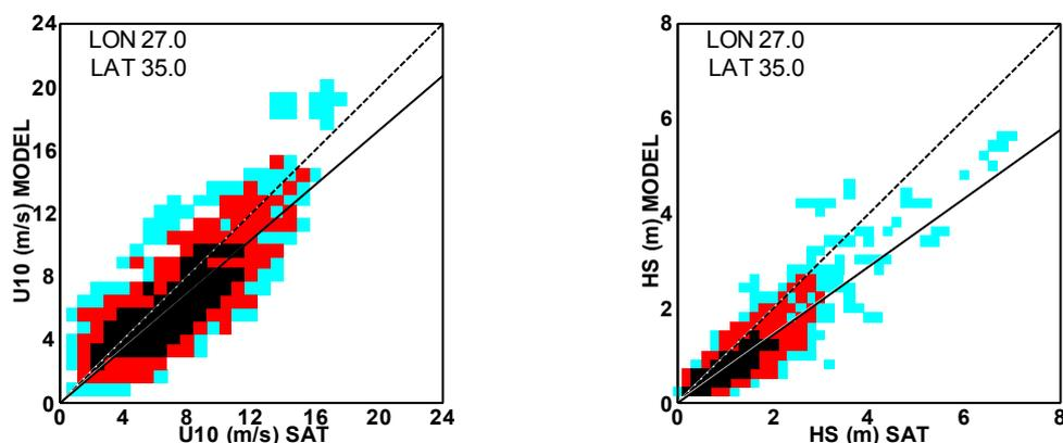
Figure 5 Scatter diagrams and best-fit lines between the ECMWF model results (surface wind speeds and significant wave heights) against Topex altimeter data at one location in the Mediterranean Sea. The considered period goes from January 1993 till June 1999. Darker pixels imply larger amounts of data.
