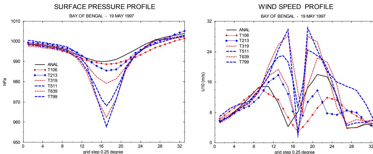
Figure 7 Upper panel: pressure distributions across a west-to-east section in a cyclone in the Bay of Bengal, according to different resolutions of the meteorological model. Lower panel: wind speed distributions along the same section.
