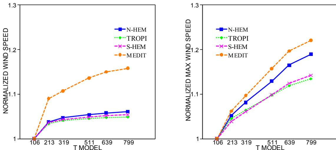
Figure 3 Left panel: relative increase of the wind speeds with the resolution of the meteorological model. Right panel: as the left diagram, but for maximum wind speeds.
