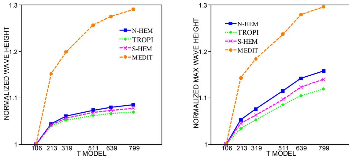
Figure 4 Left panel: relative increase of the wave heights with the resolution of the meteorological model. Right panel: as the left diagram, but for maximum wave heights.
