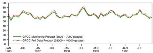
Fig. 4: Area-average monthly precipitation for the earth's land-surface for the "Monitoring Product" and the "Full Data Product" over the period Jan. 1986 to Dec. 1990.
