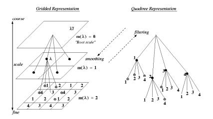
**Figure 2.** Illustration of the scale-recursive estimation (SRE) technique applied to precipitation measurements. Sparsely-distributed measurements at one scale (gray dots), and measurements at a coarser scale (solid dots), are placed on an inverted quad-tree and merged via filtering and smoothing to obtain estimates at any desired scale together with the uncertainty of these estimates.
