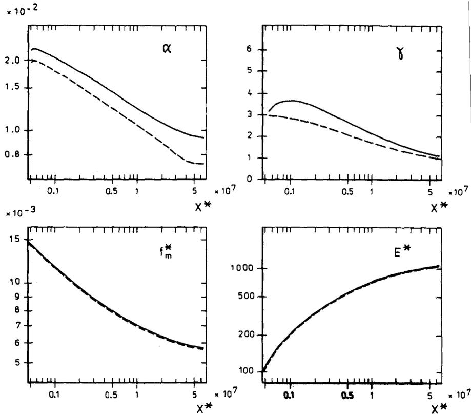
Figure 3.2 Comparison of fetch-growth curves for spectral parameters computed using the exact form and the discrete interaction approximation of  $S_{nl}$ . All variables are made dimensionless using  $u_*$  and  $g$ .
