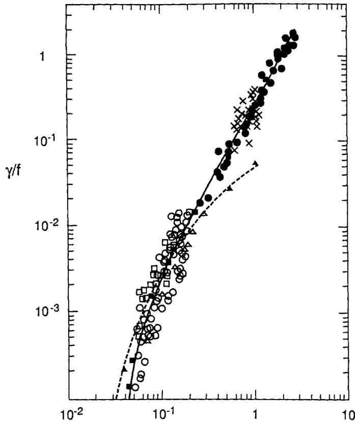
Figure 3.1 Comparison of theoretical growth rates with observations by Plant (1982). Full line: Miles' theory; full dots: parametrization of Miles' theory (3.3); dashed line: the fit by Snyder *et al.* (1981).
