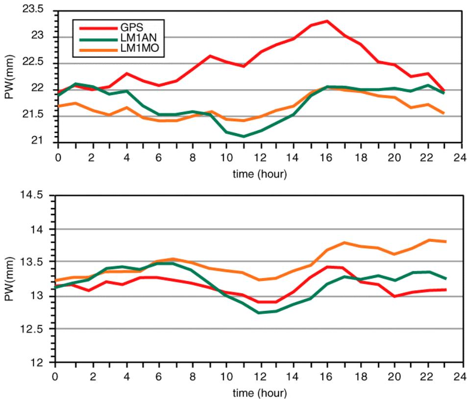
Figure 4: PW hourly average over 23 stations for the period May-August 2001 (above) and October 2001–January 2002 (below): GPS data (red), operational assimilation fields (green), 6-30 hour forecast from the 18 UTC operational forecast run (orange).
