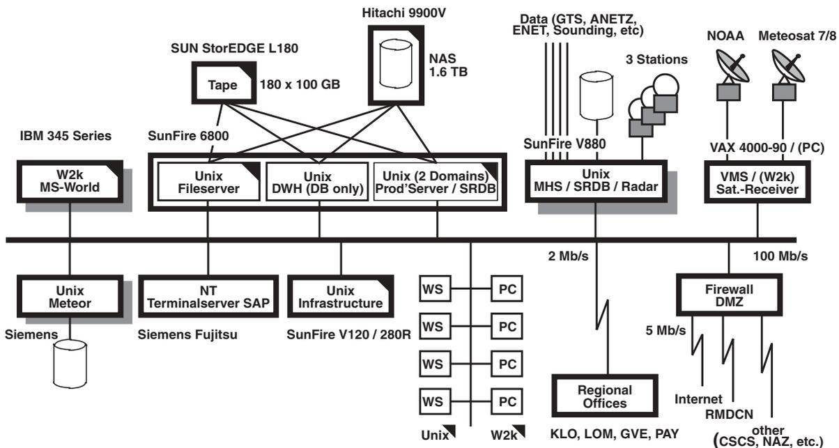
Fig 1: Configuration at Regional Offices (smaller Equipment)
