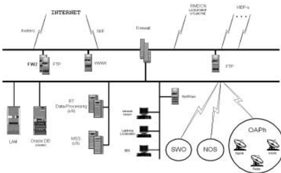
Fig. 1: HMS logical network diagram
