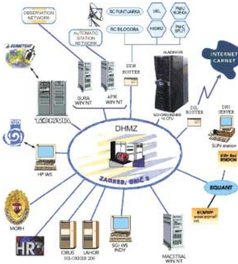
Fig. 1: Computer configuration at DHMZ
