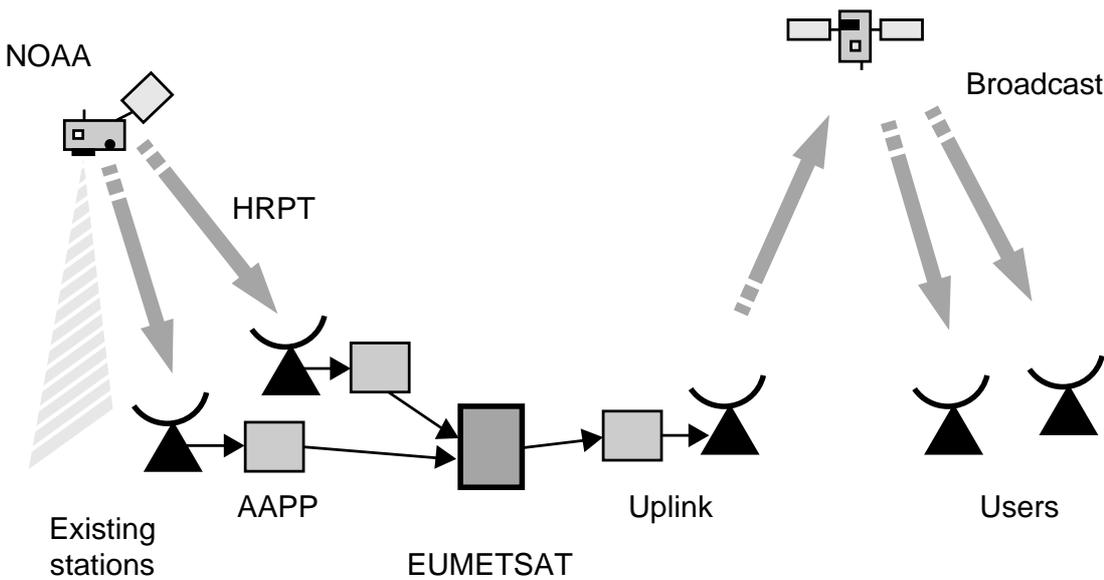
Fig. 3: The EUMETSAT ATOVS Retransmission Service (EARS) set-up.
