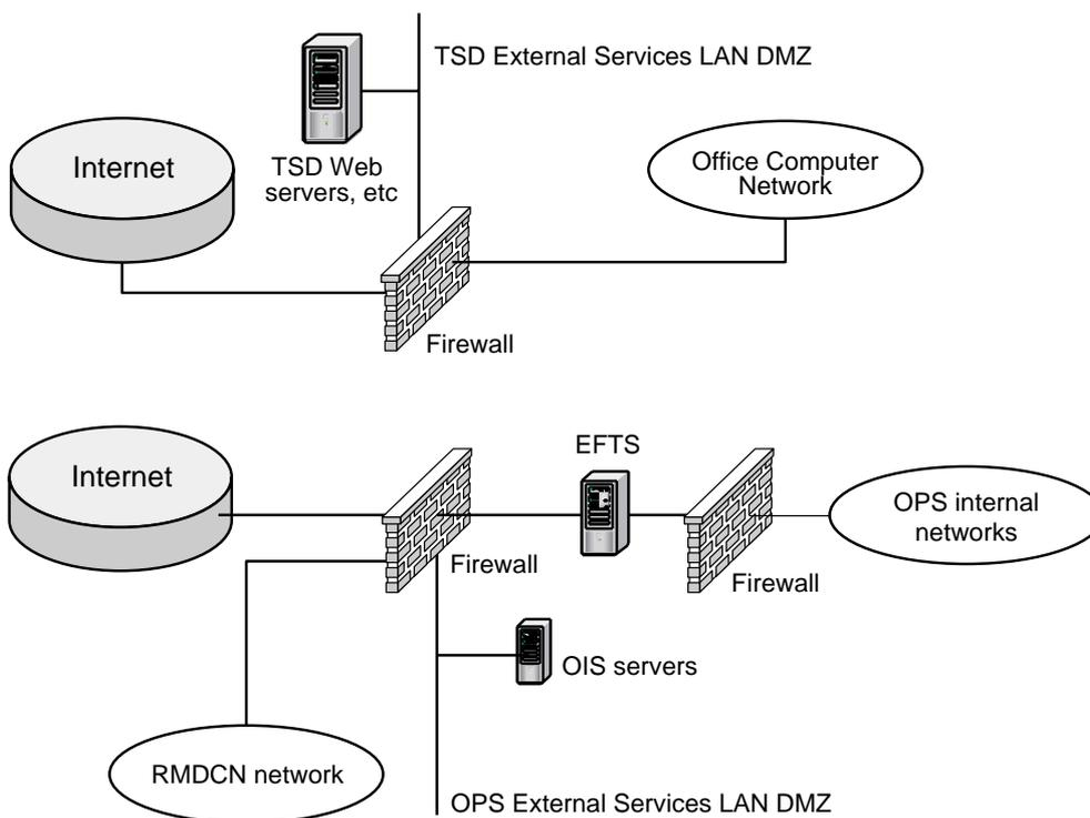
Fig. 2: The RMDCN set-up.
