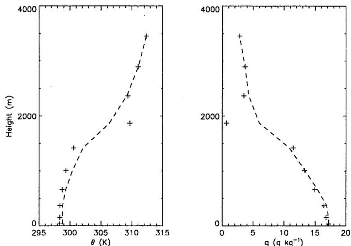
Figure 1: Potential temperature and humidity profiles obtained with the standard value of the threshold buoyancy excess. The dashed line is the initial profile, + Model profile.
