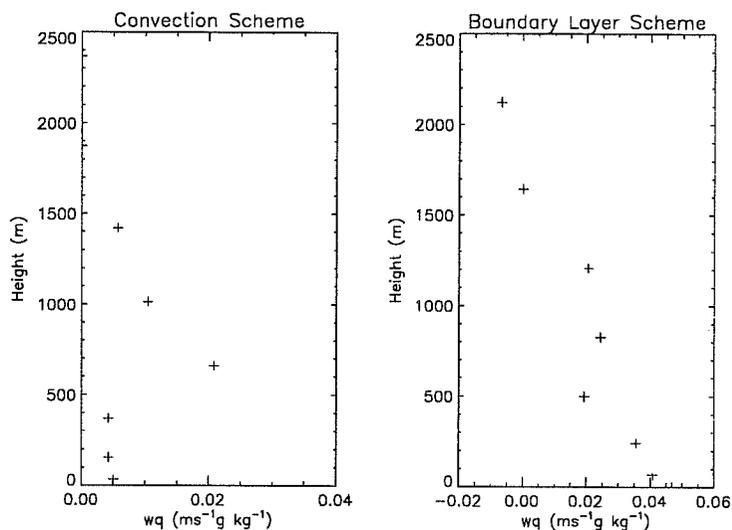
Figure 4: Moisture flux profiles diagnosed from the convection and boundary layer schemes.
