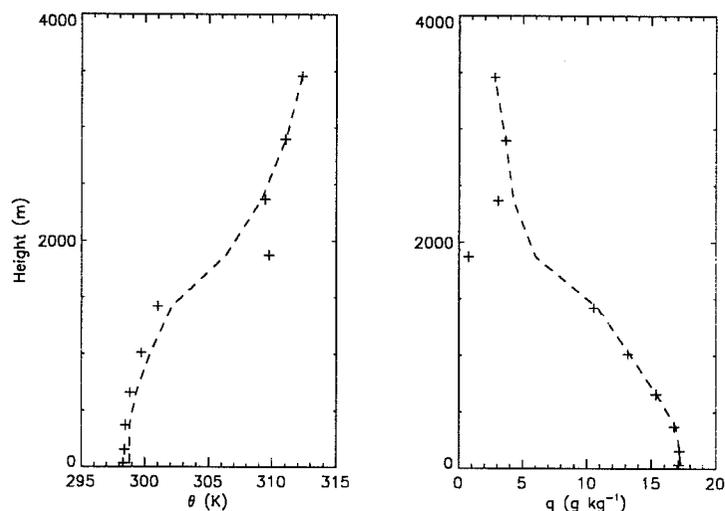
Figure 3: Potential temperature and humidity profiles obtained with a reduced value of the threshold buoyancy excess.
