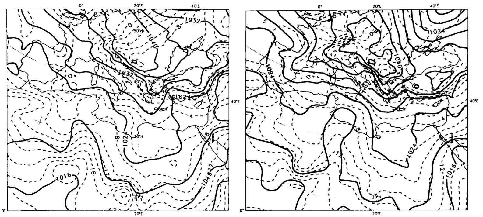
Fig. 2: MSLP (solid lines) and temperature at 850 hPa (dashed lines) for the analysis at 12 UTC 1 December, 1989 (a), and the global forecast at T+18, verifying at 6 UTC 2 December, 1989 (b). Contours every 4 hPa, and 2 degrees.
