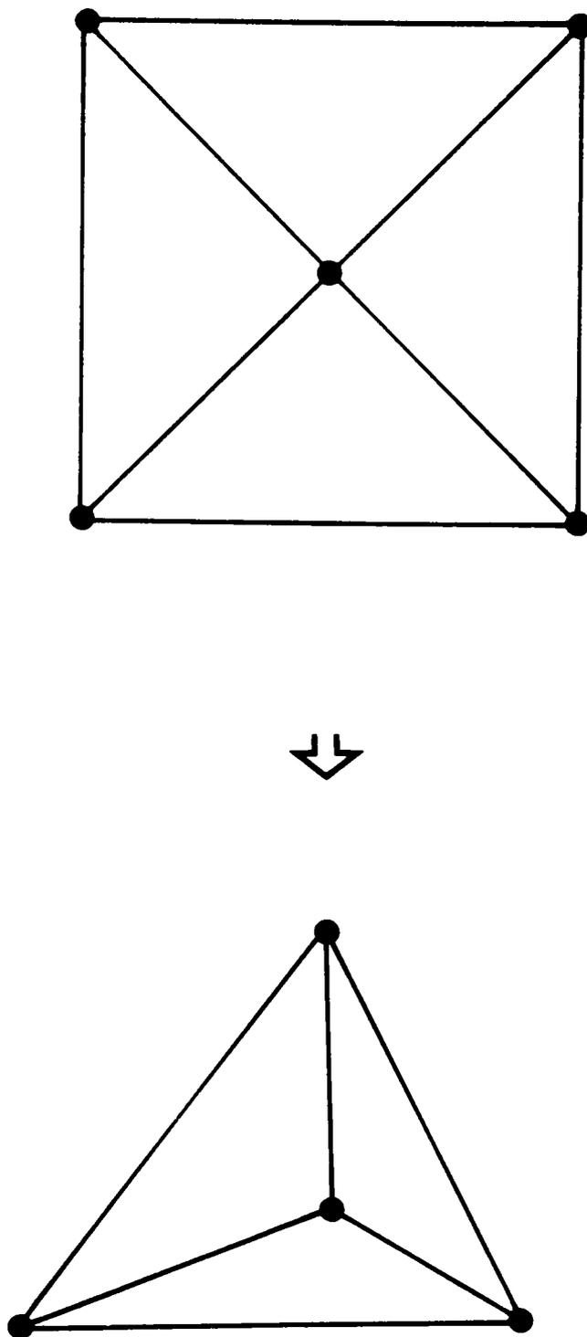
Fig. 5: A cross-bar connection between four processors is a two dimensional rendering of a simplex. In the case of four processors this is a tetrahedron.
