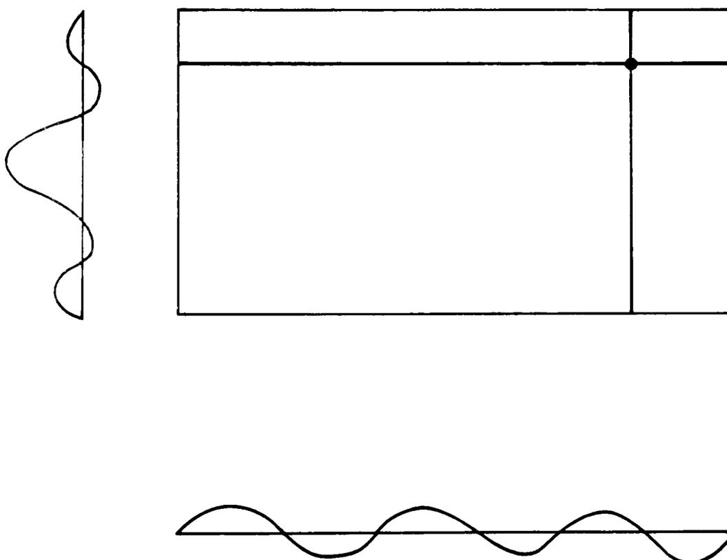
Fig. 2: A global two dimensional tensor product basis is a tensor product of two one dimensional global bases: every point is dependent on every other point on the longitude and the latitude it is on.
