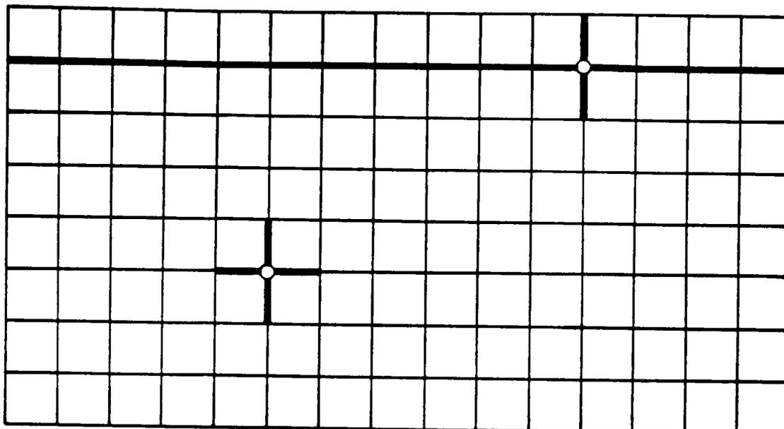
Fig. 1: Grid topology of an explicit scheme. Thick lines show data dependency patterns when the grid is mapped onto a sphere and Fourier filtering is used.
