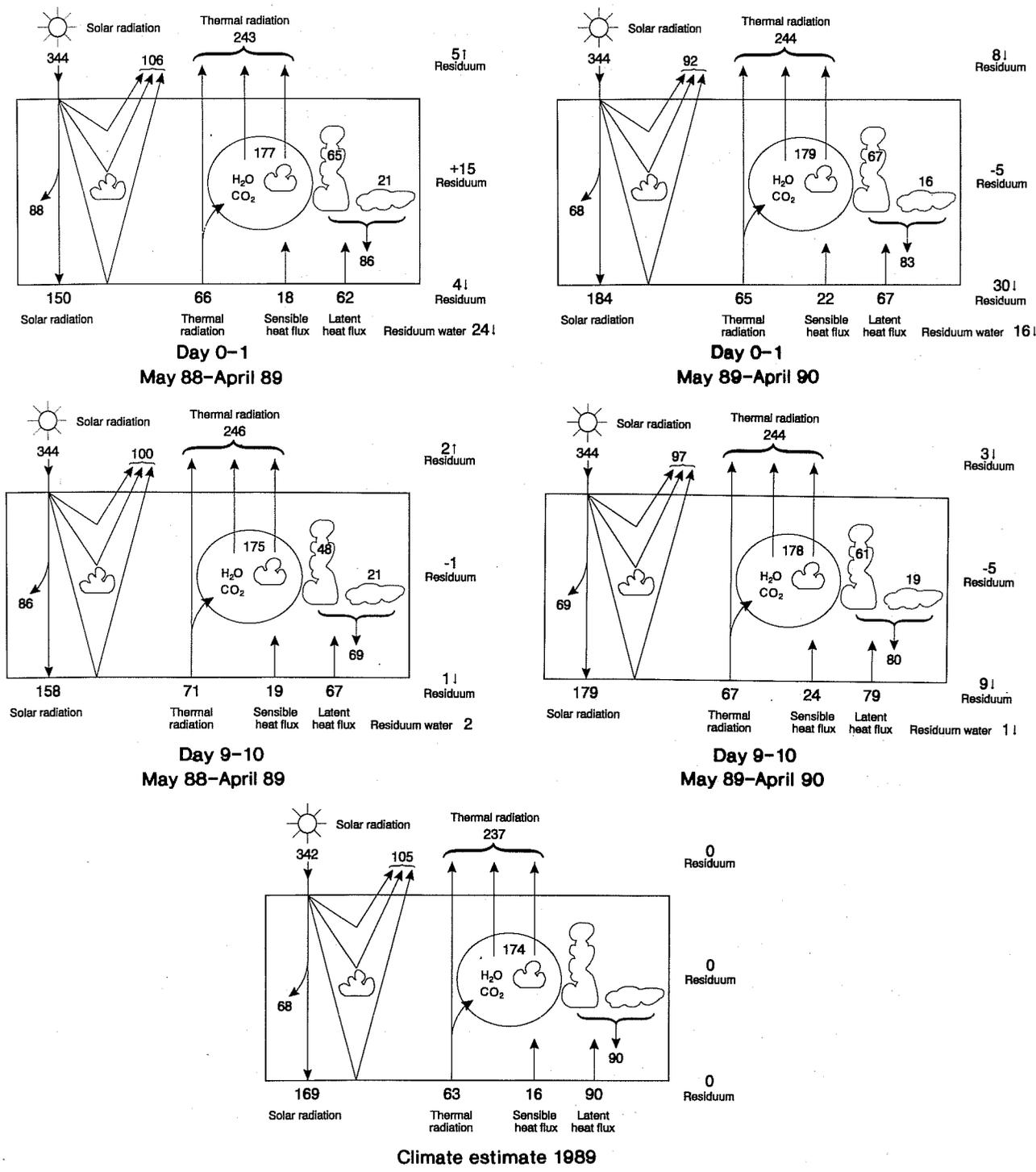
Fig. 1 Global annual mean energy and water cycle derived from day 0-1 (upper panels) and day 9-10 forecasts (middle panels) and climatological estimates of these cycles by Ramanathan et al. (1989) (lowest panel). Model data from two years with different parametrization schemes are compared. Units:  $W/m^2$ .
