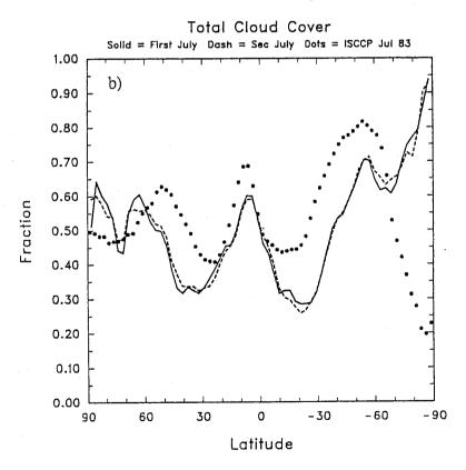
Fig. 7 Monthly mean of zonally averaged total cloud cover for a) January and b) July, solid and dashed lines CCM2, dots from ISCCP data
