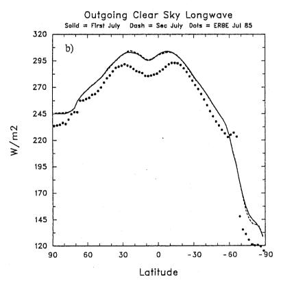
Fig. 4 Monthly mean of zonally averaged clear sky outgoing longwave flux (Wm<sup>-2</sup>) for a) January and b) July, solid and dashed lines CCM2, dots from ERBE data
