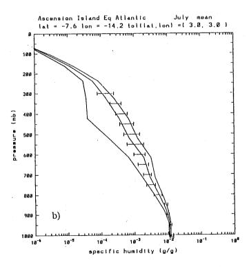
Fig. 9 Ascension island region July monthly mean vertical profiles of a) temperature and b) specific humidity, solid lines for CCM2 and horizontal bars from rawinsonde data. Central line is mean.
