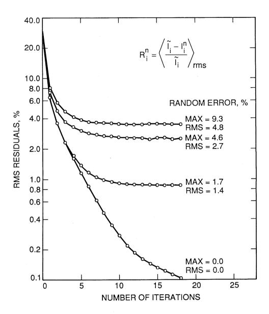
Figure 2 Residuals of the relaxation solution to a simulated set of radiances as a function of simulated noise levels and iteration. Characteristics of the radiance noise is shown for each curve.
