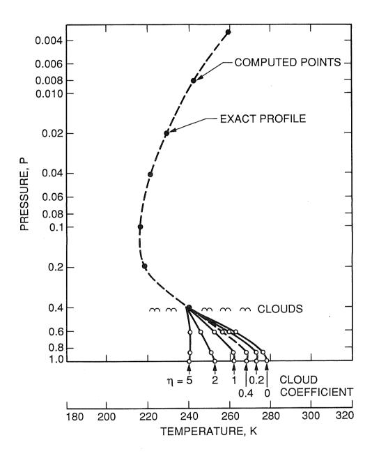
Figure 1 Clear column temperature profiles consistent with different sets of clear column radiances obtained from measurements in two fields of view assuming different values of  $\eta$ . The cloud level is indicated. Errors in  $\eta$  can produce large temperature errors beneath the cloud.
