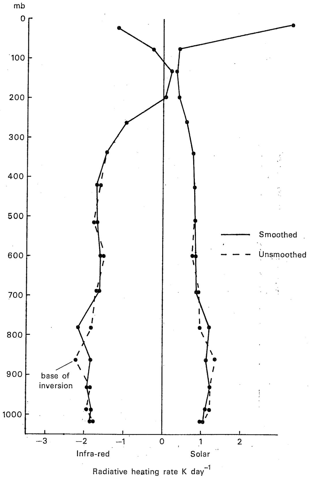
Fig. 7 Effect of vertical smoothing of humidity on the radiative heating associated with an atmospheric inversion.
