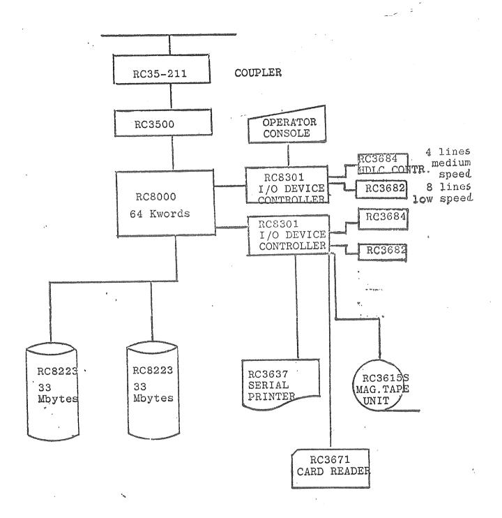
Fig. 1: The configuration of ECMWF's telecommunication system
