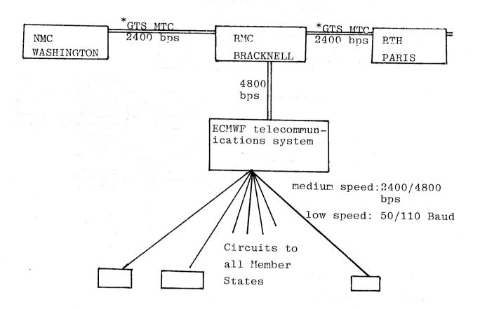
Fig. 2 : Logical structure of the ECMWF telecommunications network.
