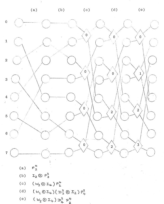
Fig. 4. The "transposed Pease" FFT for  $N=2^3$ .
