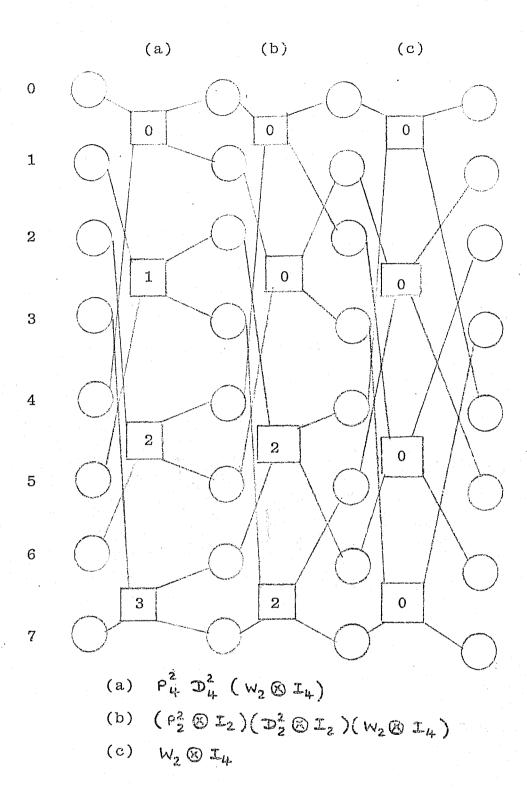
Fig. 5. Proposed new form of FFT for  $N=2^3$ .
