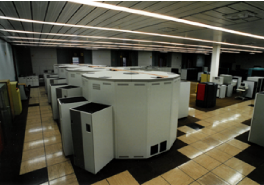
■ Figure 13: StorageTek 4400 nearline tape libraries (later rebranded to Powderhorn libraries).
