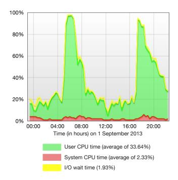
FIGURE 3 CPU utilisation on one node of ecgate on a day in 2013.
