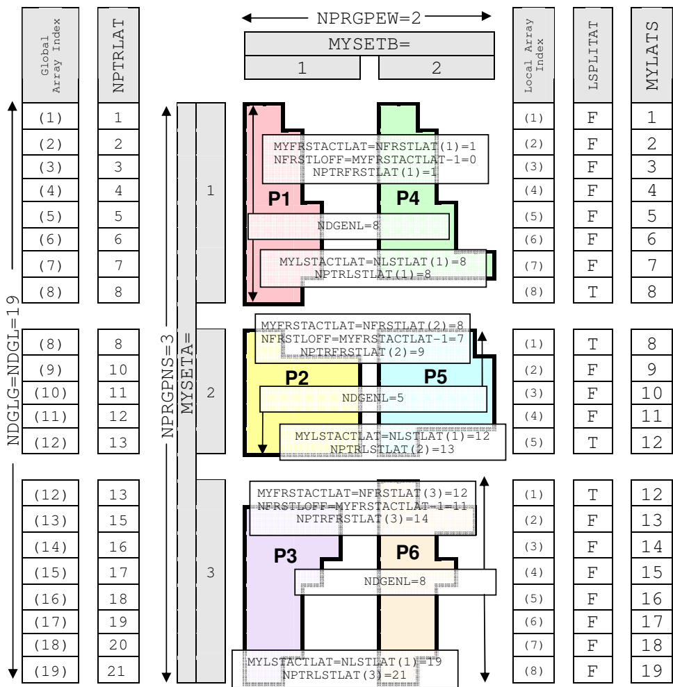
Figure 2.3 Variables describing the Grid Point Decomposition.
