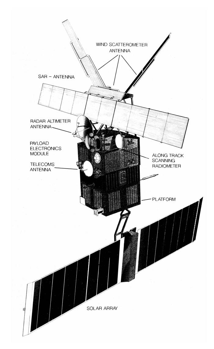
Fig. 1: The ERS-1 spacecraft (Reprinted from ESA Bulletin No. 65 - February 1991)
