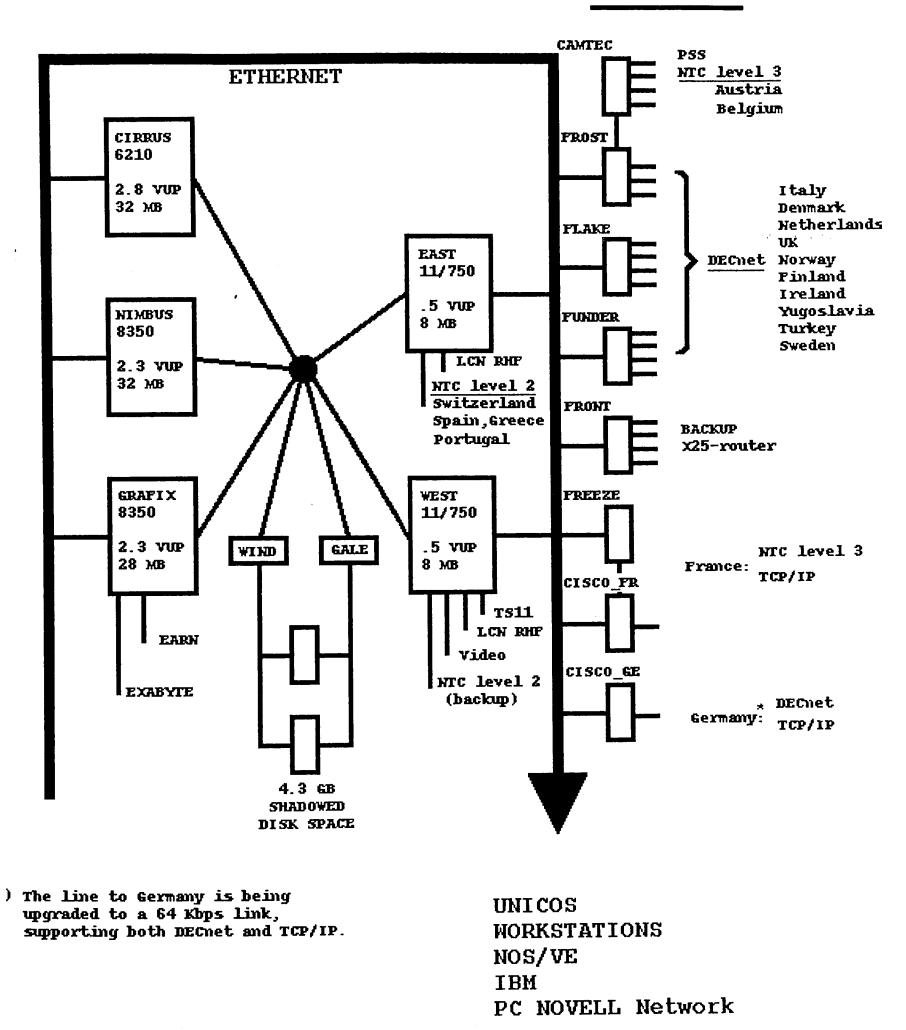
Fig. 1: Current status of the ECNET hardware configuration and the Member State connections
