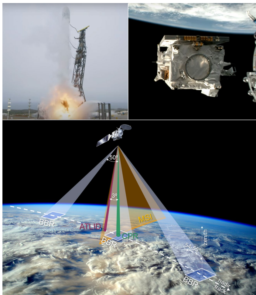
FIGURE 1 From launch to observation mode. Panels show (from top-left clock-wise), the launch of the Falcon 9 rocket carrying the EarthCARE payload; the EarthCARE satellite moments after being released into orbit; and a schematic showing the footprints of EarthCARE's four synergistic sensors (see Box A for an explanation of the acronyms). Bottom image credit: based on Illingworth et al. (2015), © American Meteorological Society, used with permission.
