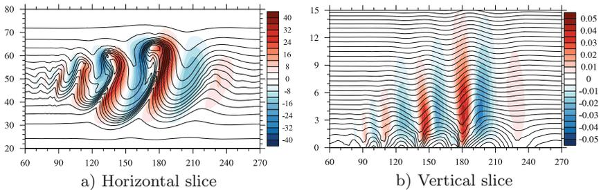
**Fig. 6.** Simulation result using hybrid finite volume module for baroclinic instability test case [10] after 8 days. (a) Horizontal slice at surface showing meridional velocity (m/s). (b) Vertical slice at latitude  $\sim 53^\circ$  N (X-axis in degrees, Y-axis in km) with shading showing vertical velocity (m/s) and solid contour lines showing isentropes (5 K interval).
