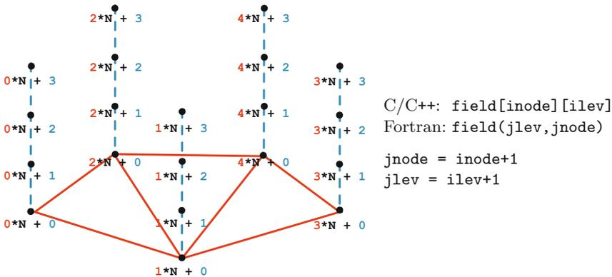
**Fig. 5.** Memory layout of a scalar field in 3D domain: solid lines show the underlying unstructured mesh; dashed lines mark the structured vertical columns with  $N$  denoting the number of vertical levels; and dots, numbered with memory offsets from the first index of the 1D array, represent the field values.
