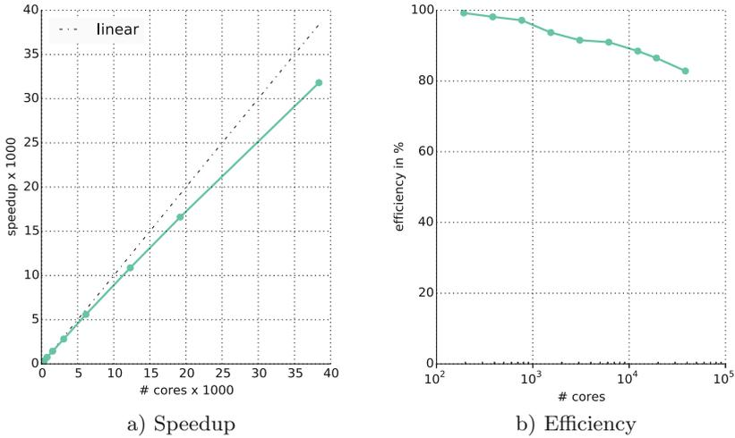
**Fig. 7.** Preliminary strong scaling results for the hybrid finite-volume module on ECMWF’s Cray XC-30 HPC. The results are created using a setup for solving hydrostatic equations, on a mesh with  $\sim 5.5$  million nodes and 137 vertical levels.
