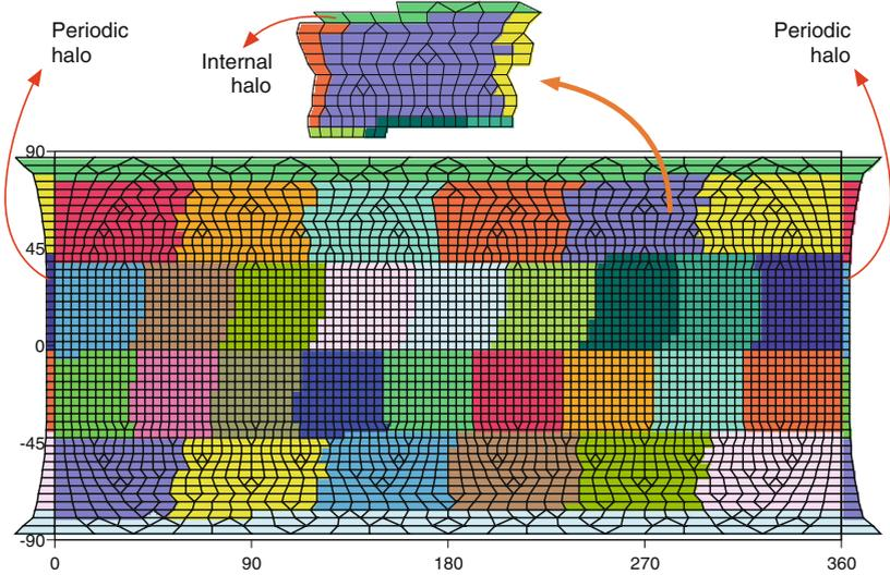
**Fig. 4.** Equal regions domain decomposition (32 partitions) for a coarse mesh with  $\sim 3500$  nodes ( $\sim 400$  km grid spacing), projected on a longitude-latitude domain. Each partition is surrounded by a thin halo. Periodicity is provided through periodic halos.
