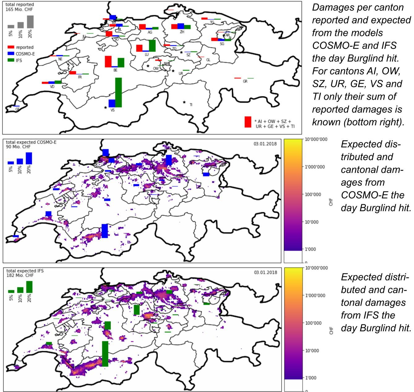
In this analysis we consider wind gust ensemble forecasts of two models, IFS and COSMO- $E^2$ , hitting Switzerland's infrastructure during storm Burglind the 3rd January 2018. The infrastructure is modelled using the LitPop model<sup>3</sup> and its vulnerability to wind storms is approximated according to Schwierz et al. 2010<sup>4</sup>. We compare the resulting damages to the ones reported by the Swiss cantonal building insurers.
