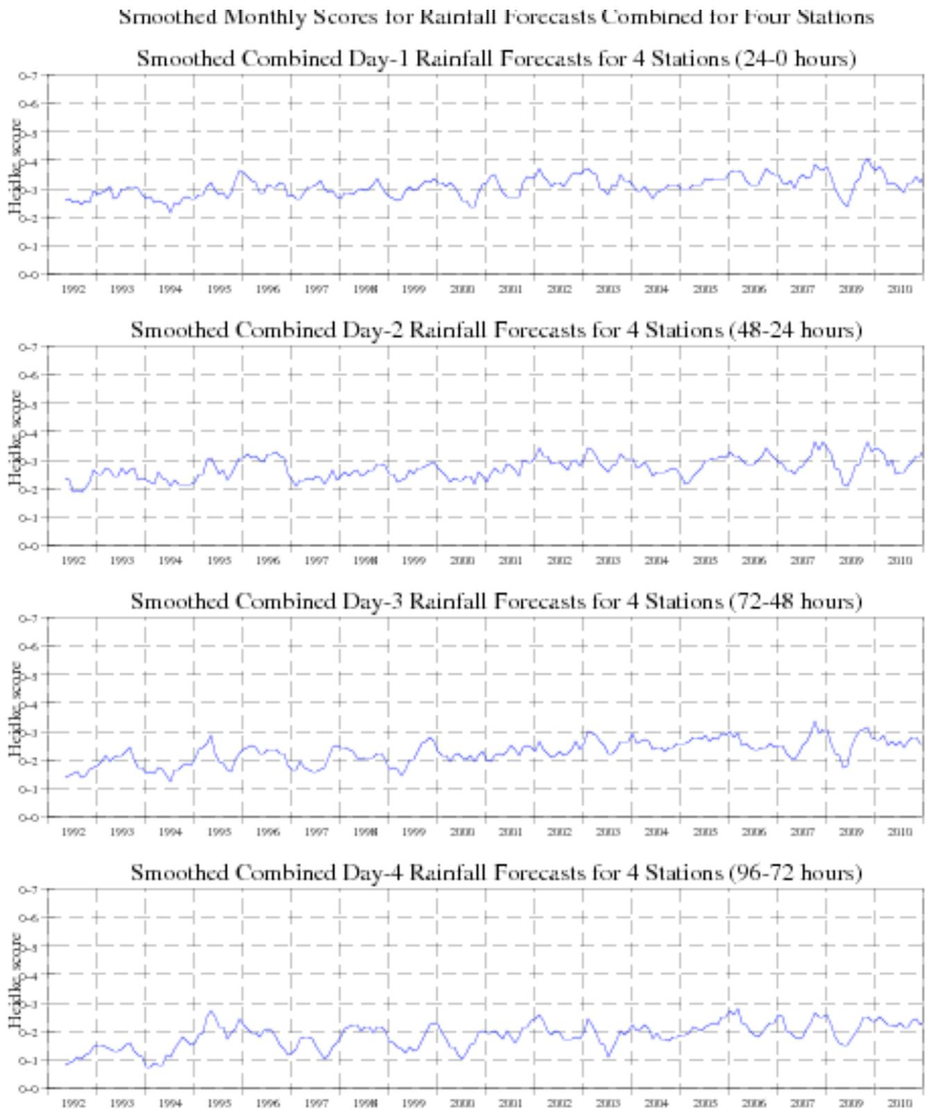
**Figure 10** Verification of precipitation forecasts: The plots show smoothed values of the mean monthly Heidke score for four stations. The smoothing is carried out by means of a 5-month centered running mean. The larger the value of the score the better the forecast. The results show that there is skill in the rainfall forecast and that the shorter forecasts are more skilful than the longer.
