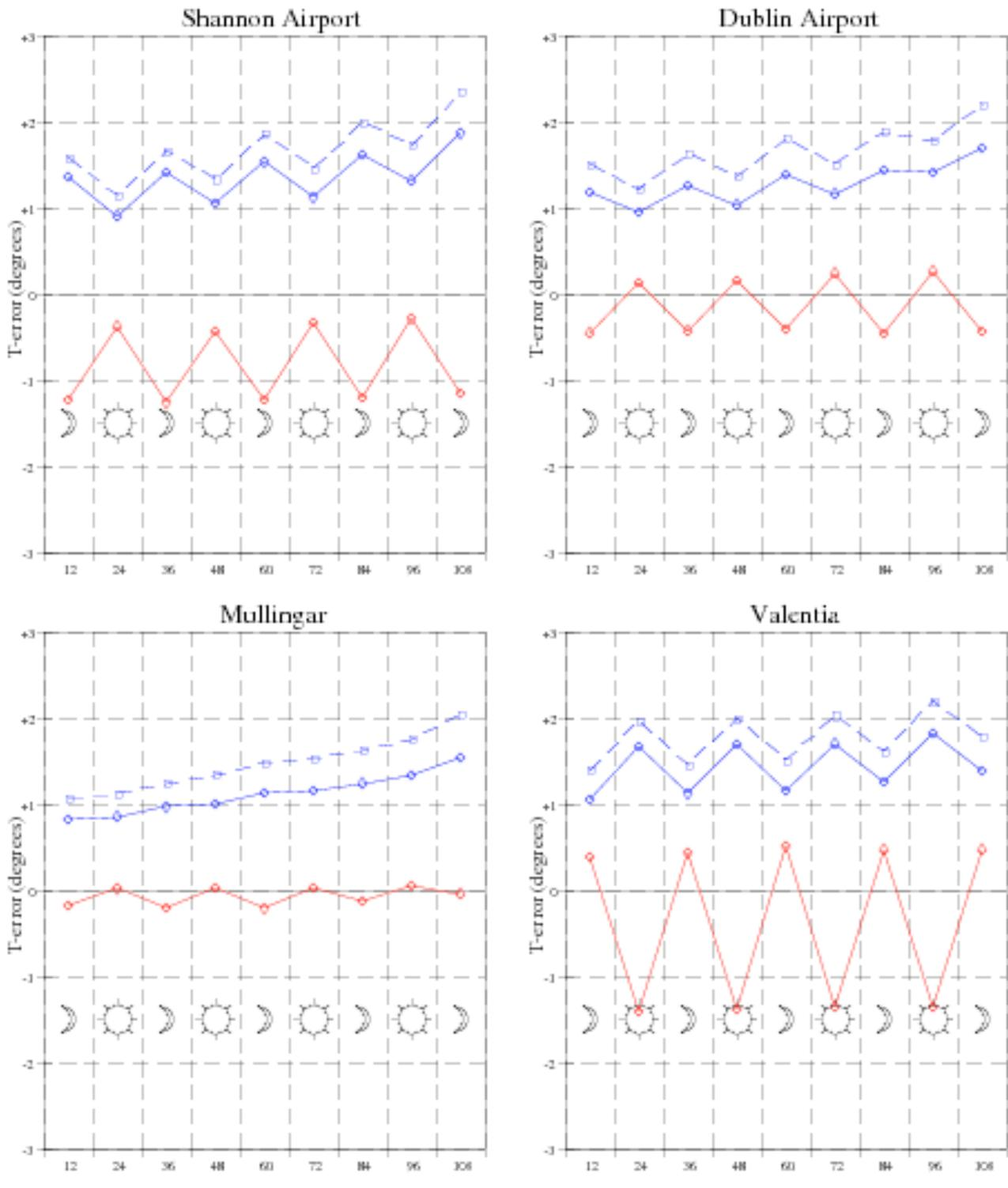
Figure 7 Mean scores for ECMWF forecasts of 2-metre Temperature, in 2008, averaged over a year of data. The solid blue line is the mean absolute error, the dashed blue line the rms error and the red line the mean error or bias. It can be seen that the quality of the forecast decreases with the length of the forecast. The 'sun' and 'moon' symbols indicate forecasts verifying at midday and midnight, respectively. The length of the forecast [in hours] is indicated on the x-axis.
