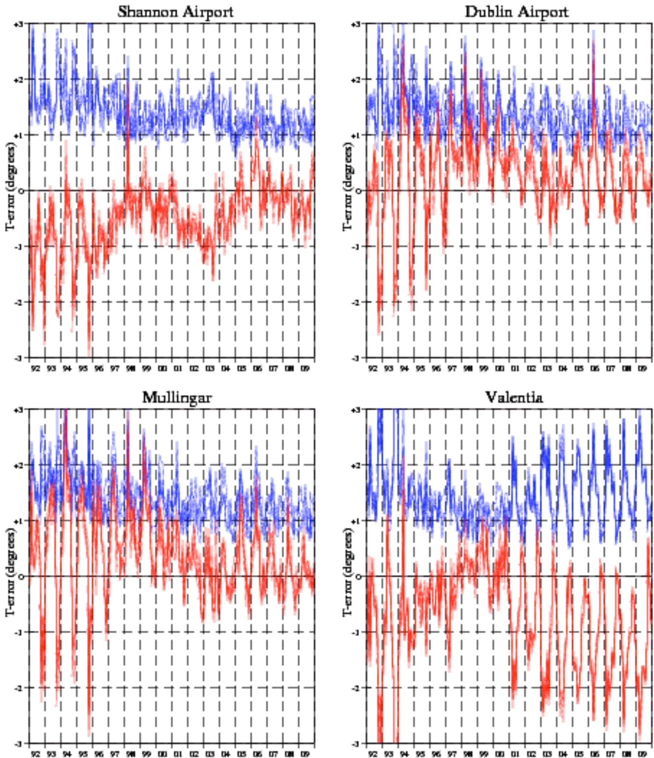
**Figure 1** Scores for the T+24, T+48, T+72, and T+96 ECMWF forecasts of 2-metre Temperature. Note that all these forecasts verify at midday. The blue lines show values of the monthly mean of the absolute error, the red lines values of the monthly mean of the mean error or bias.
