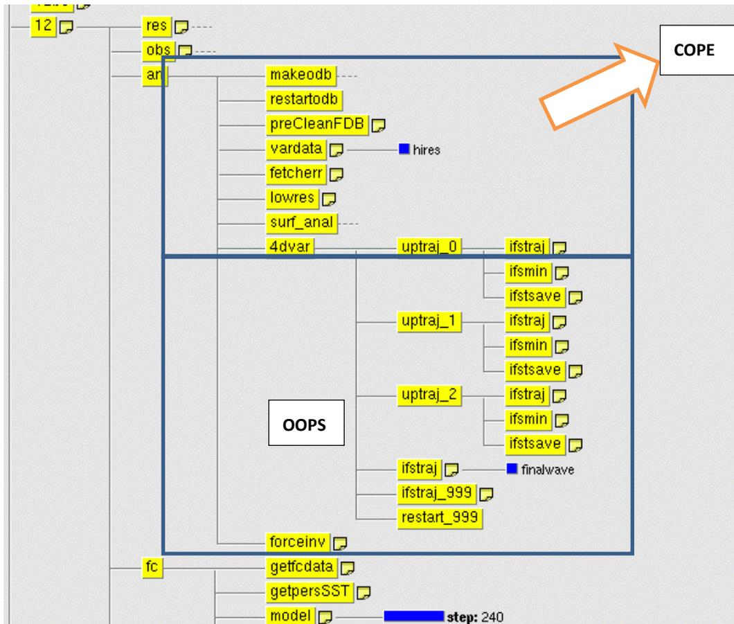
Figure 5: A schematic representation of the data assimilation tasks handled by COPE (Continuous Observation Processing Environment) and OOPS (Object Oriented Programming System) in ECMWF's next generation data assimilation system.
