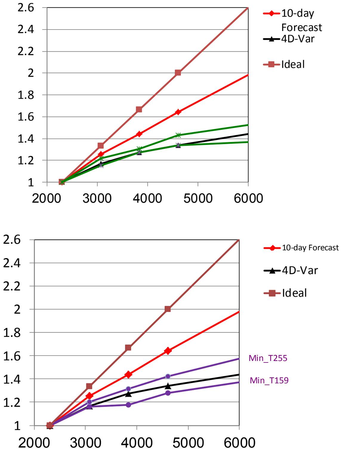
Figure 2: Scalability of the ECMWF forecast model and 4D-Var assimilation system. The upper panel include the trajectory steps (green curves). The bottom panel include the minimization steps. Speed up is shown as function of number of threads. The ideal scaling curve is also shown. Courtesy Deborah Salmond (ECMWF).
