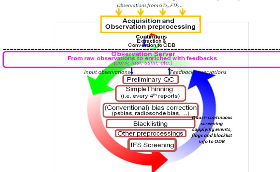
Figure 6: A schematic diagram describing the main tasks handled by the COPE (Continuous Observation Processing Environment) that is under development at ECMWF. Courtesy Anne Fouilloux.
