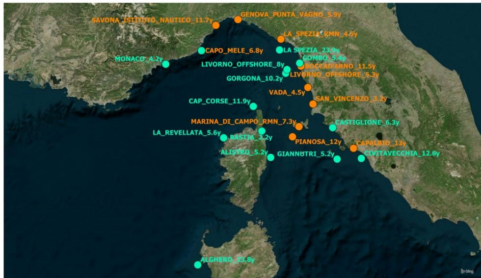
**Figure 3.** Location of wind stations (orange points) and wave buoys (light green points) used to calibrate and validate the wind/wave hindcast. The length of the time series period is shown after the underscore (“\_”) symbol following the name of the wind station or wave buoy.
