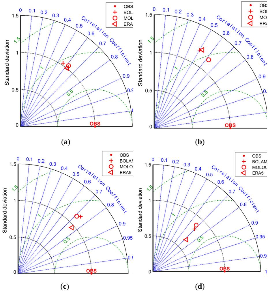
**Figure 4.** Normalized Taylor diagrams for the: (a) Bocca d’Arno, (b) Capalbio, (c) Livorno offshore and (d) Vada wind stations. The plus (+), circle (○) and triangle (△) symbols refer to the BOLAM, MOLOCH and ERA5 data, respectively.
