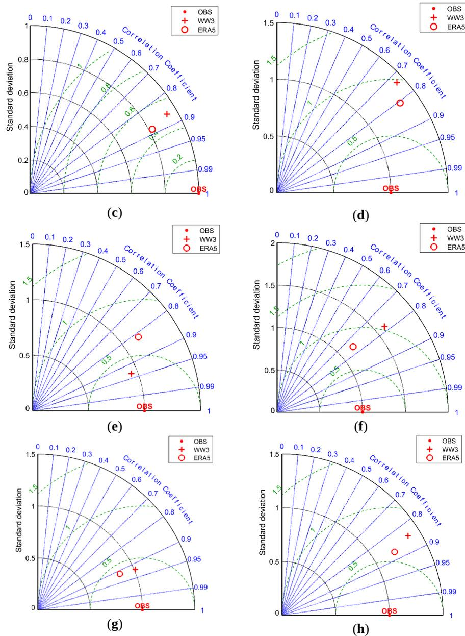
**Figure 5.** Normalized Taylor diagrams for: **(a,b)** the Bastia, **(c,d)** Capo Mele, **(e,f)** Castiglione, **(g,h)** Giannutri buoys. The results are relative to Hs **(a,c,e,g)** and Tm **(b,d,f,h)**. The plus (+) and circle (○) symbols refer to the wave hindcast (here WW3) and ERA5 data (here ERA5), respectively.
