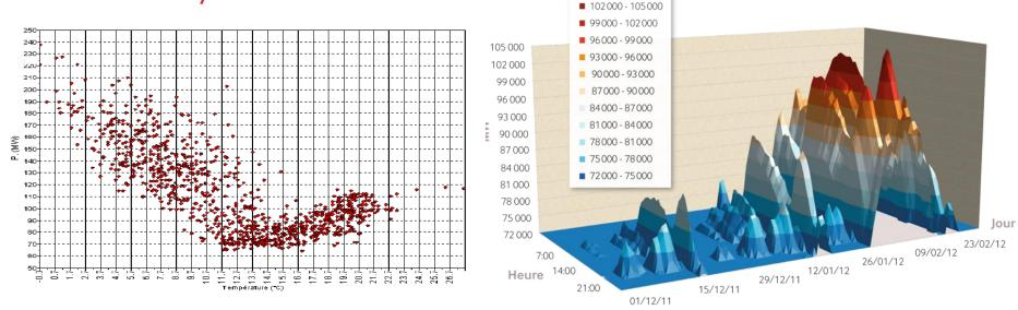
France : ~2400MW/Celsius Degree in winter Consumption for cooling in summer is increasing ⇒ Accurate temperature forecasting is required (deterministic/probabilistic)
