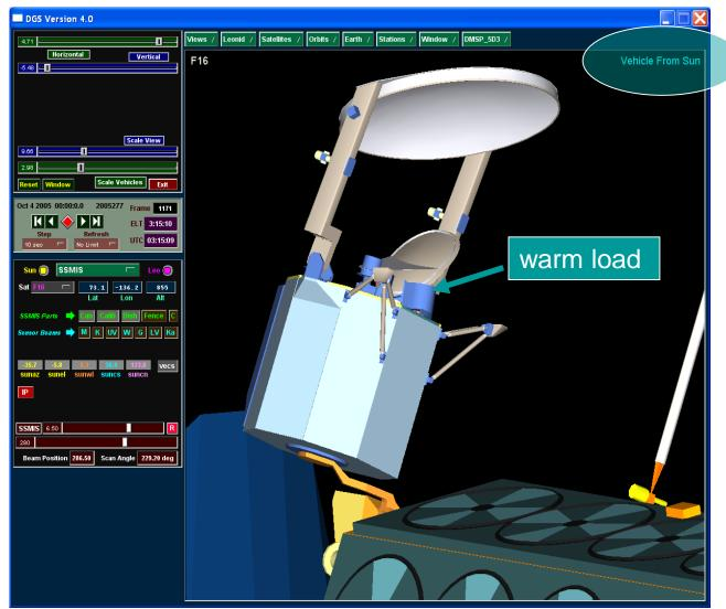
For F-16 - 3 or 4 times per orbit solar radiation illuminates warm load tines, through:
