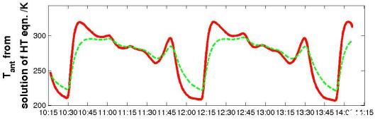
Reasonable agreement with temperature evolution derived from solving the heat transfer equation
