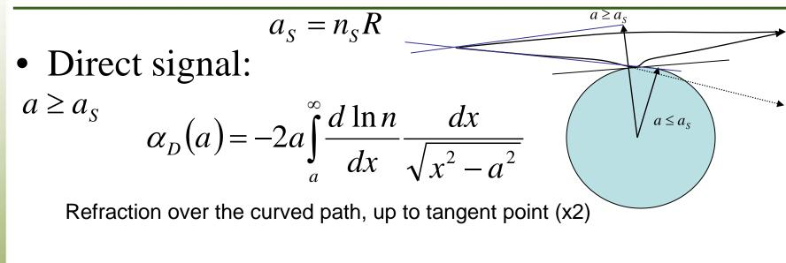
• Reflected signal:  $a \le a_{S}$   $\alpha_{R}(a) = -2a \int_{a_{S}}^{\infty} \frac{d \ln n}{dx} \frac{dx}{\sqrt{x^{2} - a^{2}}} - 2 \arccos\left(\frac{a}{a_{S}}\right)$ Nearly always downwards (>0) Upwards (<0) Impact parameter that is tangent at surface
