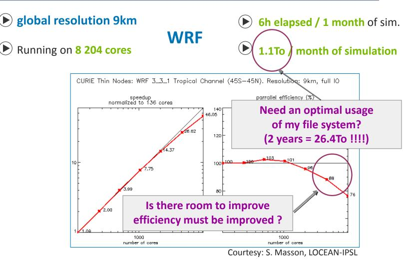
76% of parallel efficiency on 8 204 cores (based on 136 cores run)
