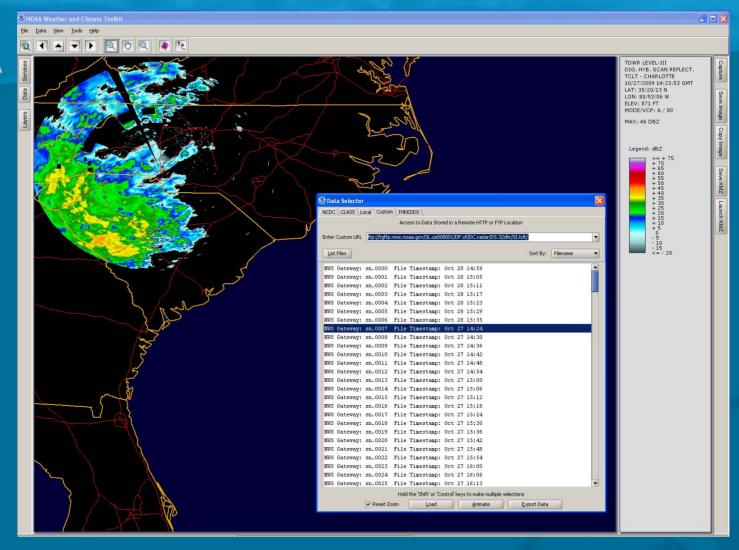
TDWR data displayed in toolkit using near real time data accessed from NWS server
