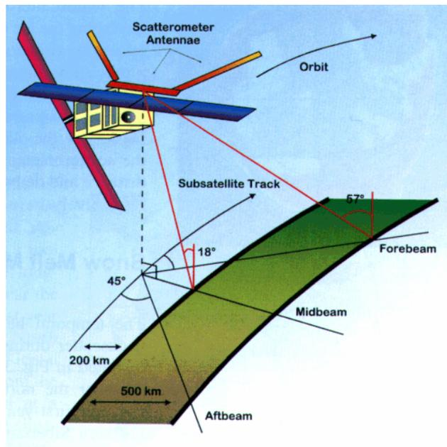
Figure 5. Illustrating the viewing geometry of the AMI scatterometer.
