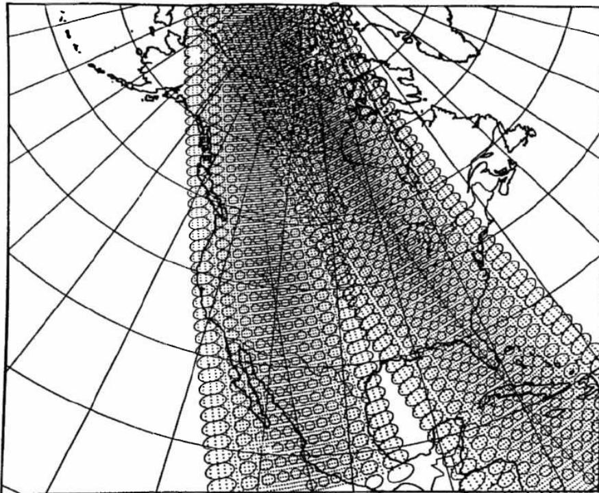
Figure 1: TOVS scan patterns for HIRS (small dots) and MSU (larger ellipses), from Smith et al. (1979).
