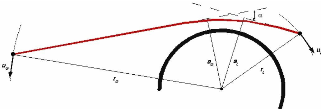
Figure 8: The geometry of a radio occultation measurement showing the refracted ray from a transmitting satellite (on the left) to a receiving satellite (on the right).
