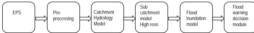
*Figure 2 A possible flood forecasting cascade, showing a cascade of components. Note that not every flood modelling system driven by EPS will have exactly these components; this remains an example, and we have purposefully not included other possible downstream components such as ‘warning dissemination’ and ‘coordination of flood protection measures’ as these are beyond the scope of this review.*
