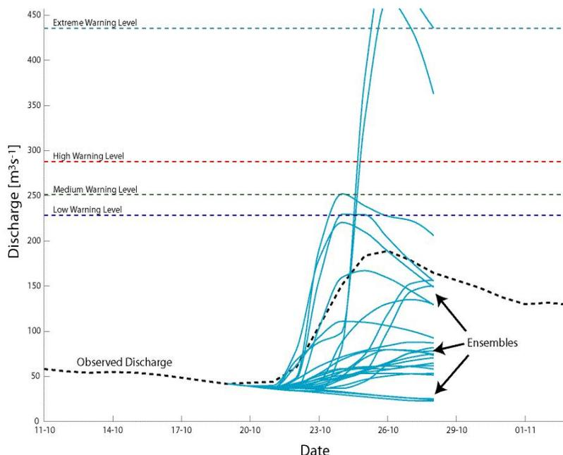
Figure 1 An example of an ensemble spaghetti discharge hydrograph plot for a hindcasted flood event. The plot shows the discharge predicted for each ensemble forecast (solid line), the observed discharge (dashed black line) and four flood discharge warning levels (horizontal dashed lines).
