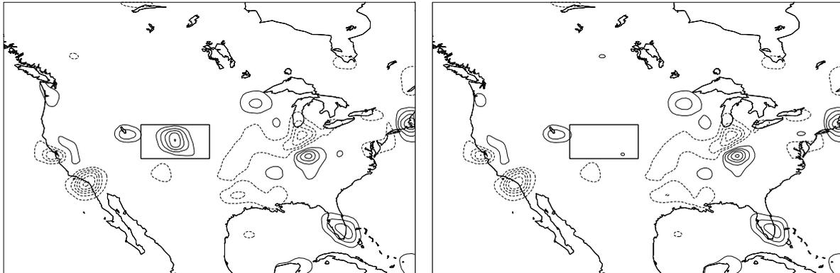
Figure 11: Average temperature forcing at the lowest model level over North America, with all data on the left, without aircraft data in the area shown on the picture on the right. Contour interval is 0.01 K/h.
