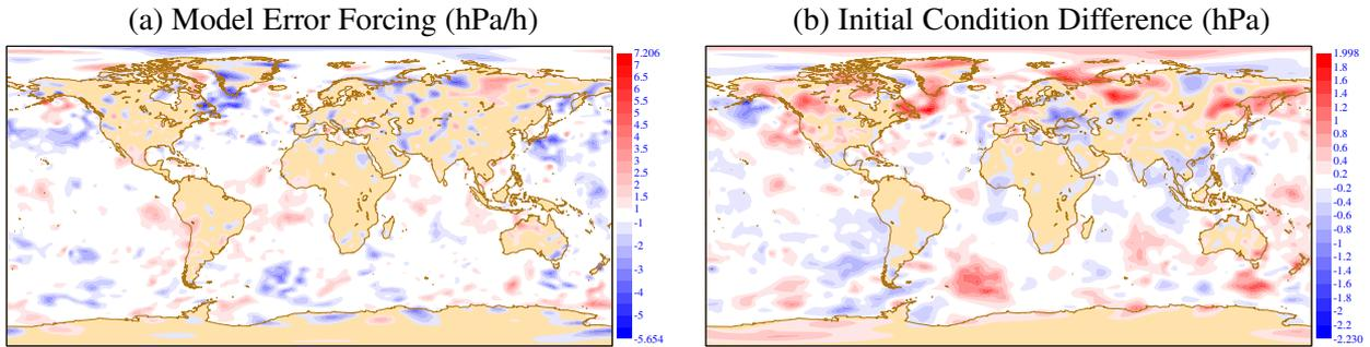
Figure 2: Surface pressure model error obtained with constant forcing and  $Q = 10^{-1}B$  on 01-05-2004 at 0UTC on the left. The corresponding change in the initial condition increment is shown on the right.
