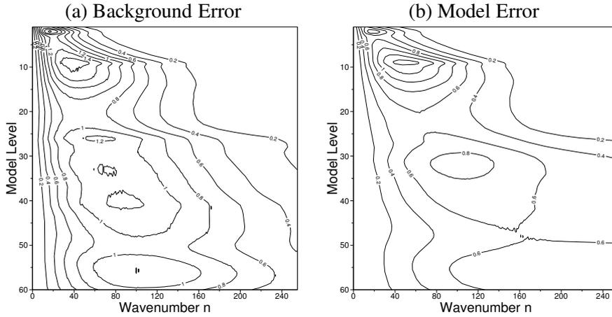
Figure 5: Divergence background and model error standard deviations as a function of wavenumber. Values are scaled by a factor of  $10^{-6}$  and contour interval is 0.2 for both figures.
