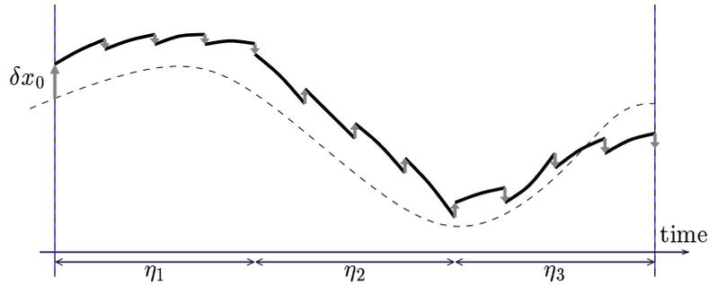
Figure 1: Weak constraint 4D-Var with model error forcing control variable. In the schematic example presented here, the forcing is constant for each of three intervals in the assimilation window (denoted  $\eta_1$ ,  $\eta_2$  and  $\eta_3$ ). It is applied at every time step, for illustrative purposes four times in each interval.
