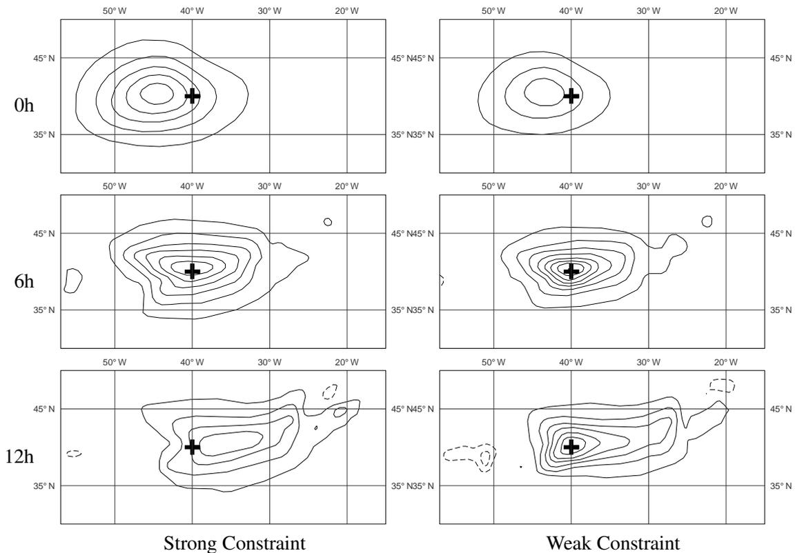
Figure 6: Evolved temperature increments for strong and weak constraint 4D-Var with temperature observations at every hour, located at 40N, 40W (as marked by the + sign) and with departures of 1K. Contour interval is 0.1K.
