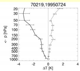
Break profile is calculated at 00GMT, 12GMT at breakpoints. Adjustment only if 90% significant and larger than 0.3K at two p-levels at least Data to estimate adjustment: 1-8 years, depending on interval between breaks
