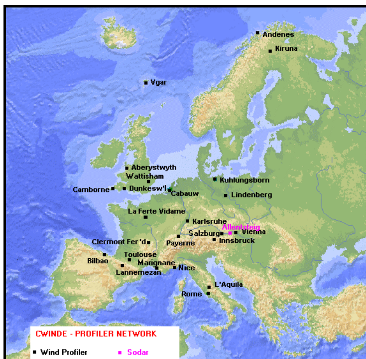
Figure 1 The European wind profiler network. The map is from the web site of the CWINDE-99 project, coordinated by the MetOffice.
