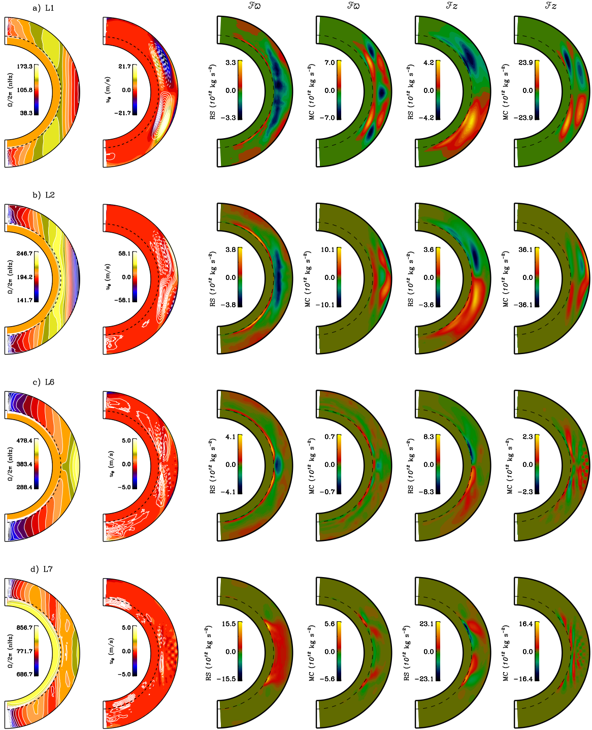
Fig. 3.— Differential rotation, meridional circulation (panels 1 and 2 from left to right in each row) and angular momentum flux components of Eq. (13): \mathcal{F}_\omega^{RS} , \mathcal{F}_\omega^{MC} , \mathcal{F}_z^{RS} and \mathcal{F}_z^{MC} (panels 3 to 6 from left to right), for the simulations L1, L2, L6 and L7 (top to bottom). All the profiles correspond to mean azimuthal value averaged over \sim 3 years during the steady state phase of the simulation.
